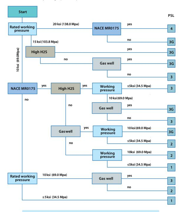
For special services such as Surface safety (SSV), Blowdown (BDV) or Shutdown systems, Velan suggests a minimum level of PSL 2, while for Boarding shutdown (BSDV) and High-integrity pressure protection system (HIPPS) the minimum level should be increased to PSL 3.
