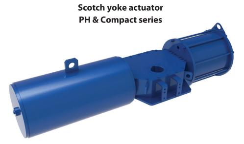
We have extensive experience in the design and manufacturing all types of scotch yoke actuators for on/off or emergency shut down and blowdown services. The scotch yoke design provides peak torque at the break and end point of the stroke, ensuring maximum reliability and is available in both symmetric and canted designs to meet specific application requirements.
